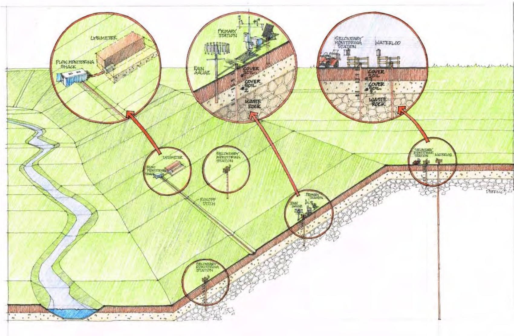
Figure 8-4. Conceptual schematic of a direct cover system field performance monitoring system for a mine waste landform.
