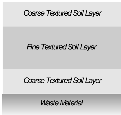
Figure 2.6 Multi-layer cover system over waste material.
